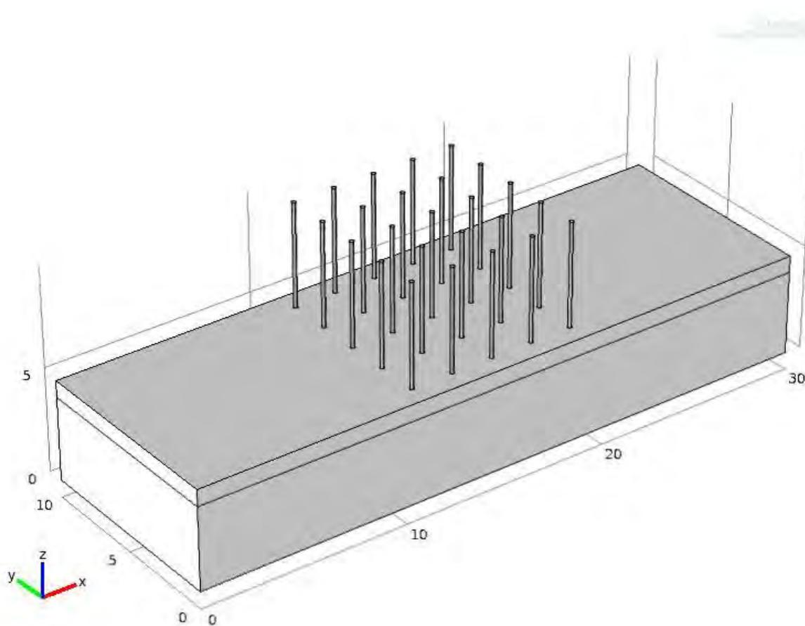
Fig: SAW Sensor with Nanowire as the Sensing Material
