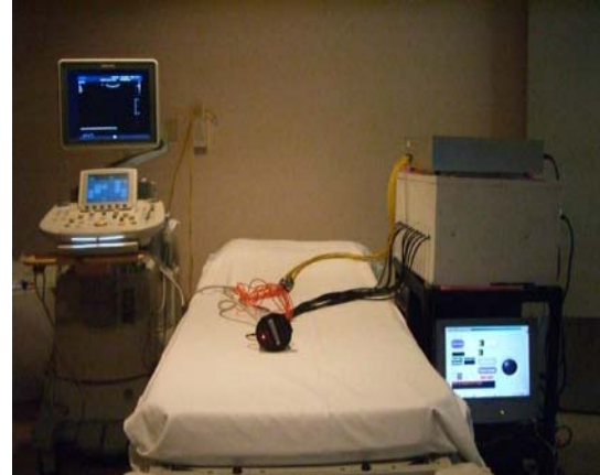
Figure 3. The ultrasound-guided NIR imaging system in the operating room
