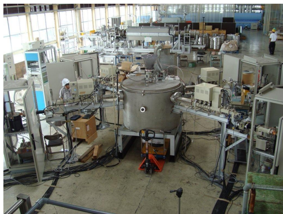
Figure 1 MW Steel Making. This furnace can make 120 kg pig iron per day [1].
