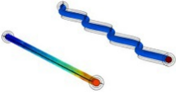
Figure 1: Concentration profile of urea post dialysis in straight and crimped fibers of hemodialyser
