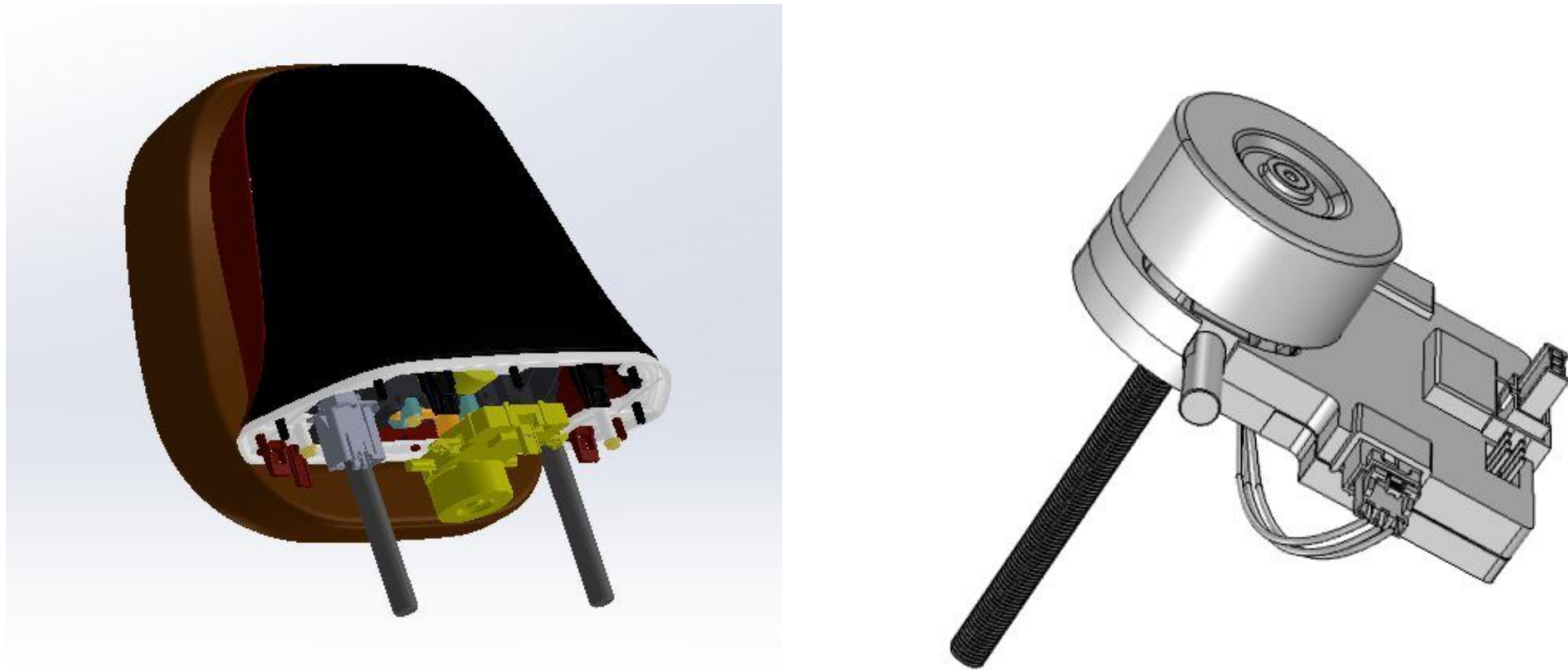
Figure 1. Head restrain module and the motor with controller
