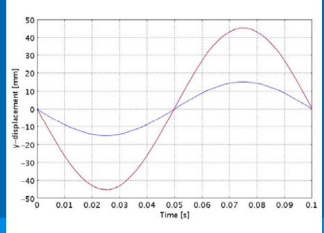
Kinematic analysis shows excellent relation between inner and outer race displacement value (the only difference between the two points is due to different radial position)
