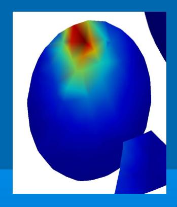
Stress distribution shows a typical pattern derived from rigid bodies contact stress (Hertzian contact) in which the maximum mean value is located under the body's surface.
