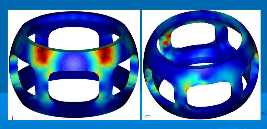
Stress distribution in the cage is very peculiar and reflects this component's typical failure mode
