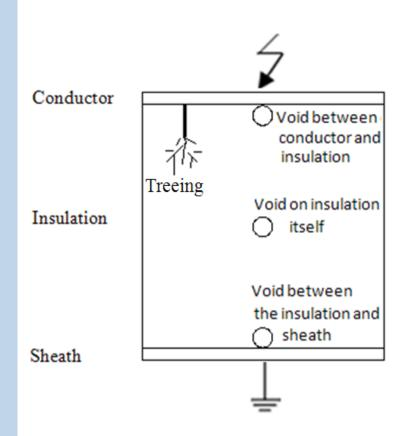
PD is a localized electrical discharge that only partially bridges the insulation between conductors which may or may not occur adjacent to a conductor.
