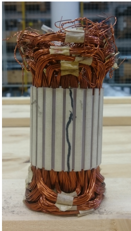
Hand-wound deflection coil prototype from the 90s
