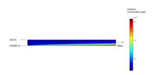
**Figure 1**: Sediment concentration in a soil pipe section. The pipe section is 1 meter long and the radius of the pipe is 0.05 m. The velocity was specified as 1 m/s on the left boundary and pressure (p=0) specified on the right boundary. The dynamic viscosity for water was specified as 0.001 Pa-s. The suspended sediment concentration is given in mg/l. The pipe wall is at r=0.05 m. The result given for the case where turbulence is absent.
