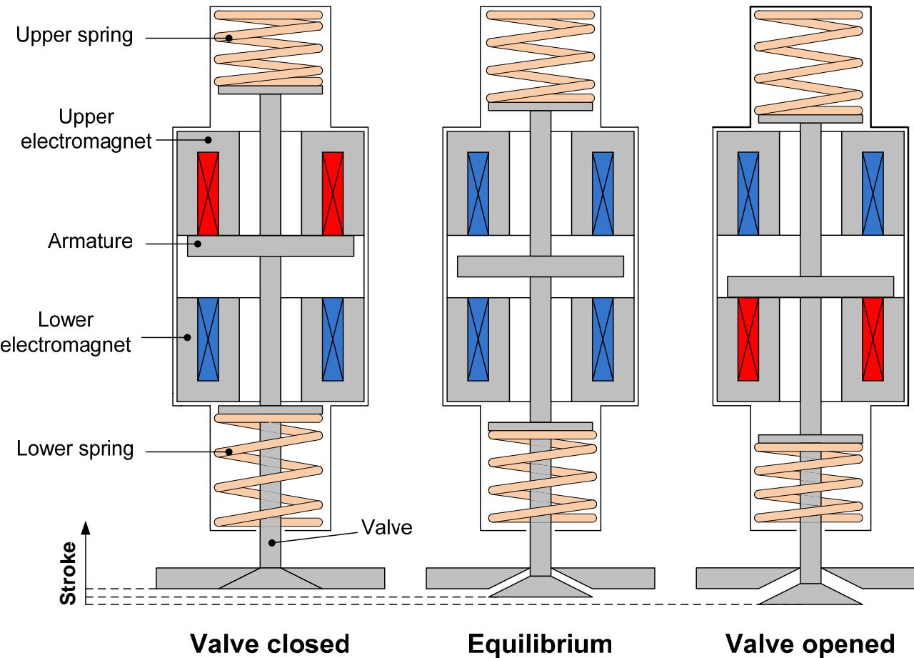
Opening and the closing events can be shifted with respect to the crankshaft angle
