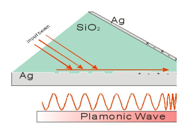
A Wave travelling along the interface between metal and dielectrics.
