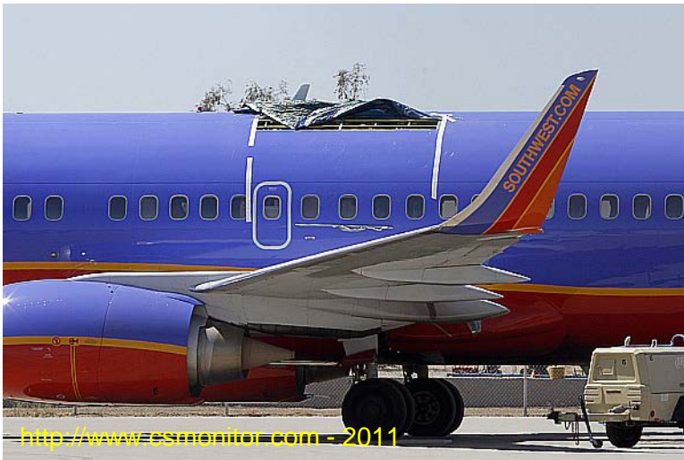
Effects of fatigue cracking in airplanes
