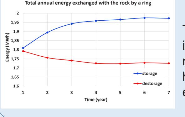
The amount of heat injected into the rock is always higher than that extracted from it.
