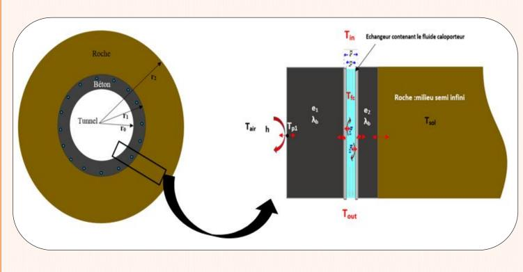
In winter, the heat pump restores the heat collected to heat buildings on the surface, and the reverse operation in the summer (cooling).
