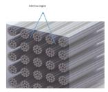
Figure 1: Schematic representation of inter-tow region in a CFRP composite laminate.
