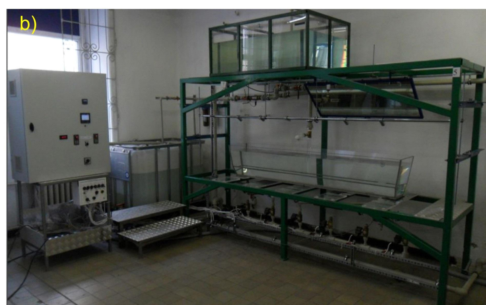
Figure 1. a) Scheme of the tundish, b) The test stand of CSC plant water model
