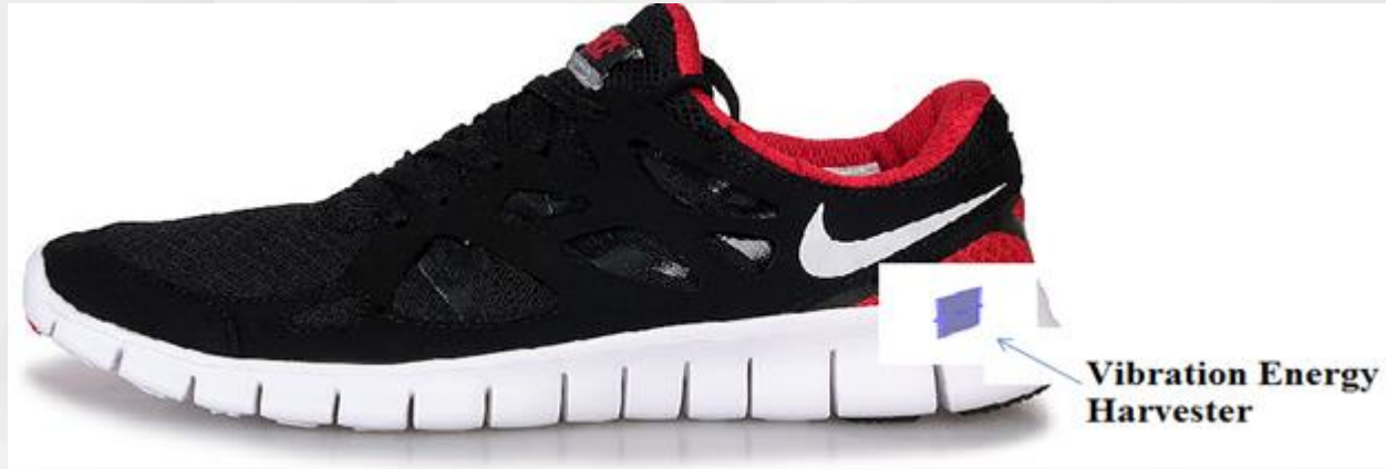
Shoe with vibration energy harvester inserted in its sole
