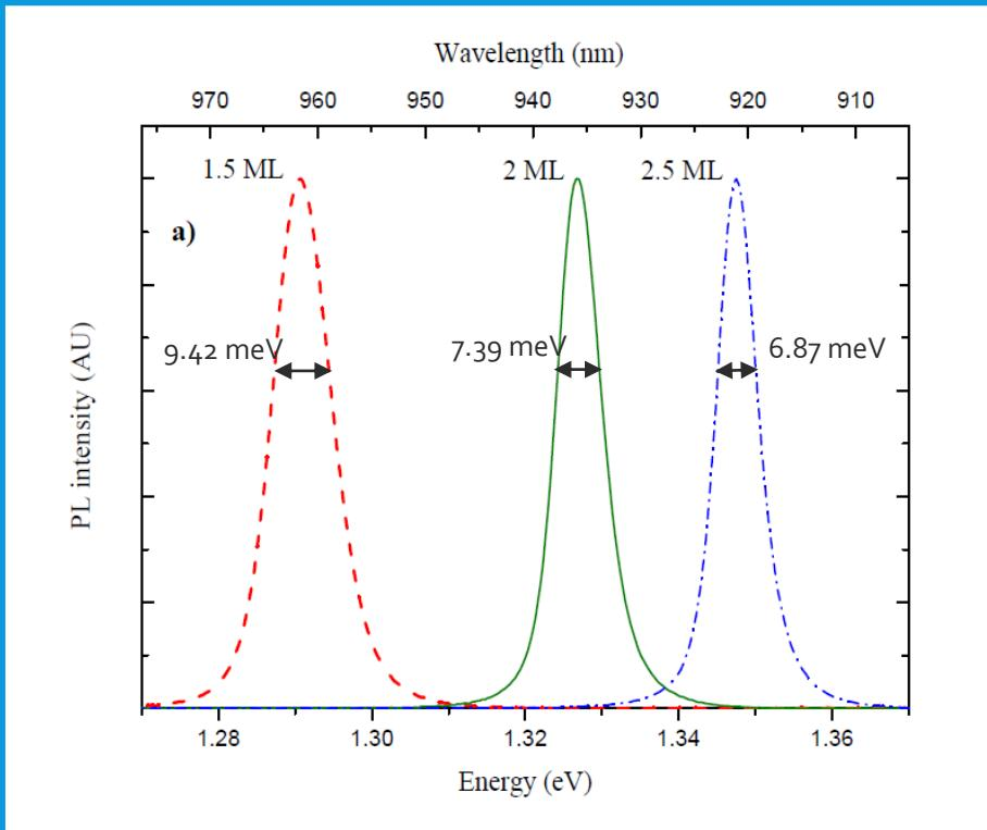
Narrow line-widths (more akin to an InGaAs QW<sup>1</sup>).
