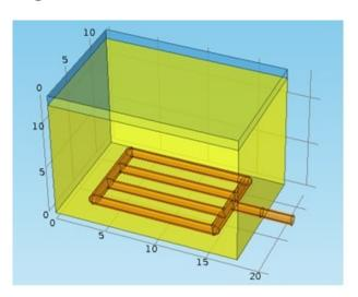
Figure 1: Schematic representation of the mash tun home brewing reactor.
