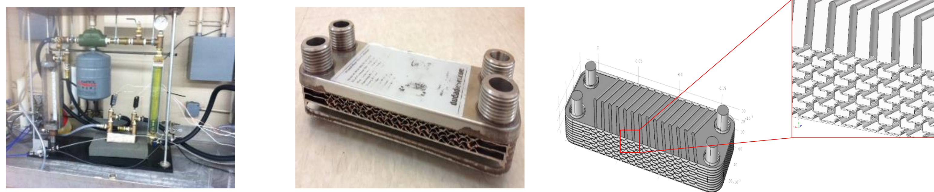
Figure 1. Plate heat exchanger experiment, cut away view of exchanger, and SolidWorks model.
