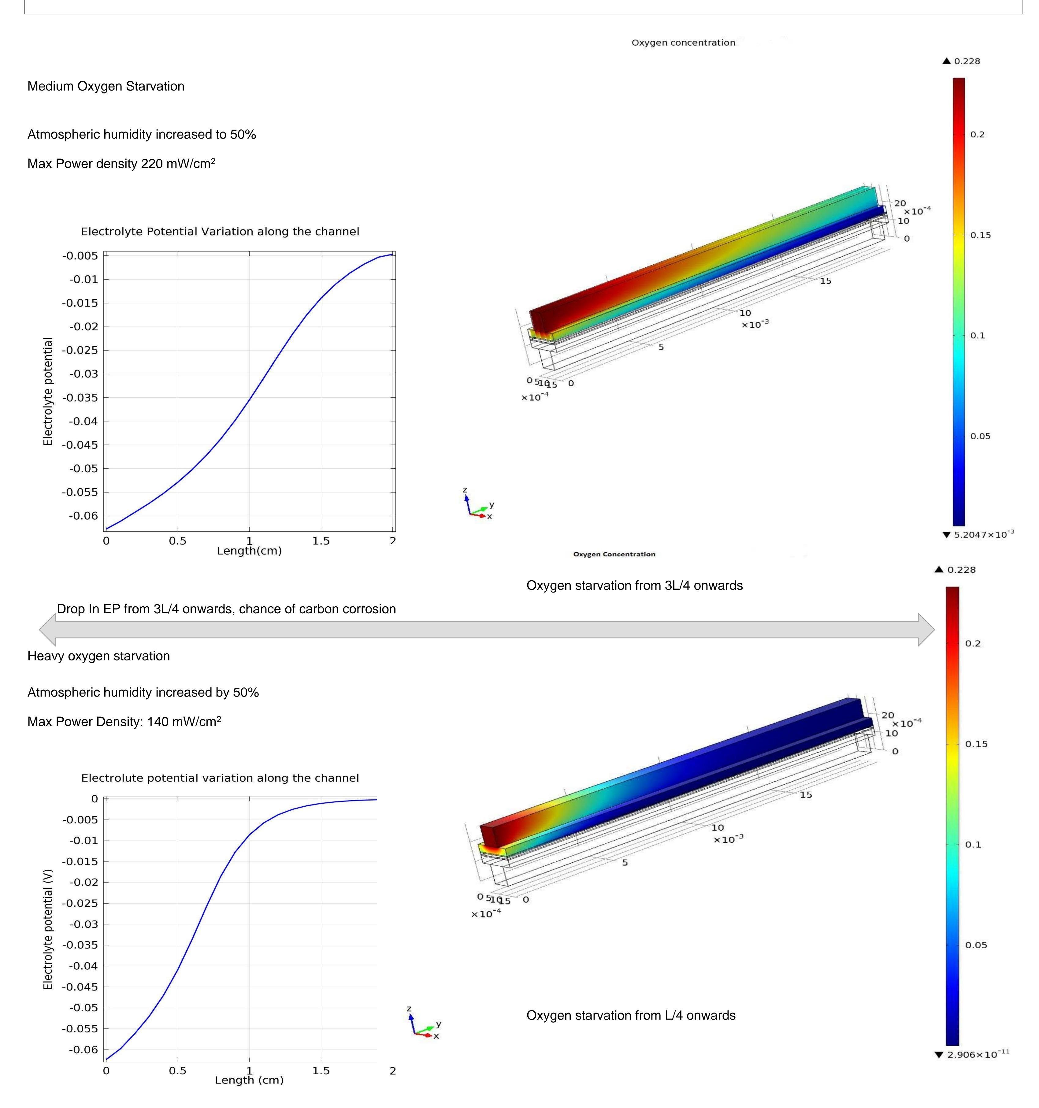
Drop in EP from L/4 onwards, high chance of carbon corrosion
