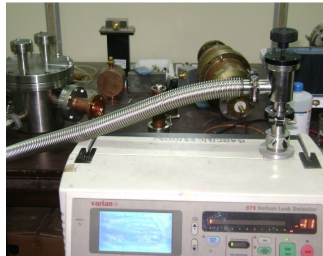
RF Coupler leak tested at LEHIPA, BARC
