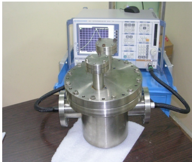
RF Cavity developed for Coaxial Coupler Conditioning
