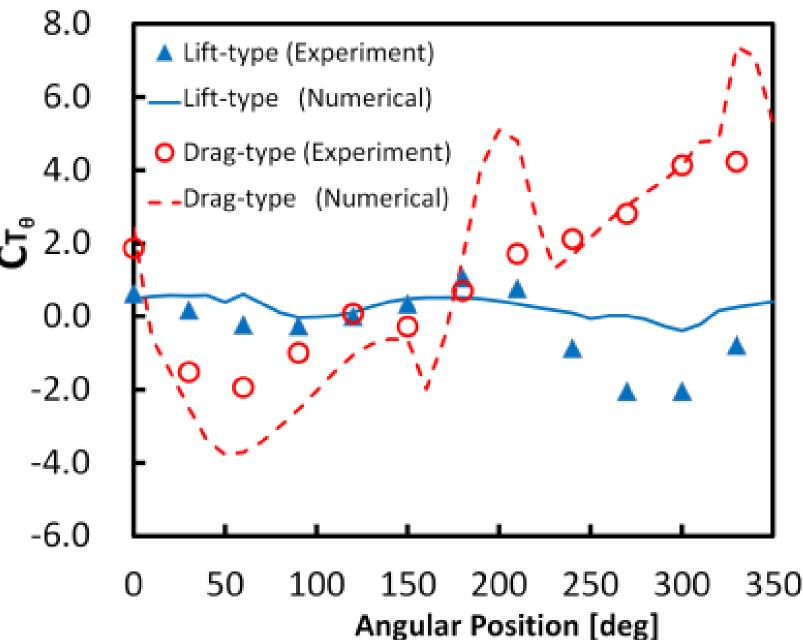
Results obtained by experiments  $(\blacktriangle, O)$  and numerical simulations (solid and broken lines) agree qualitatively.
