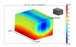
Figure 1: Fuel cell stack temperature distribution with heat pipe design.
