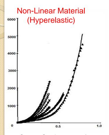
Stress-Strain curves for potatoes at different moisture contents (Krokida et al., 2000)
