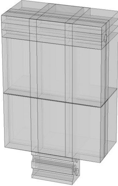
Figure 4. Geometry used for the COMSOL Multiphysics model.
