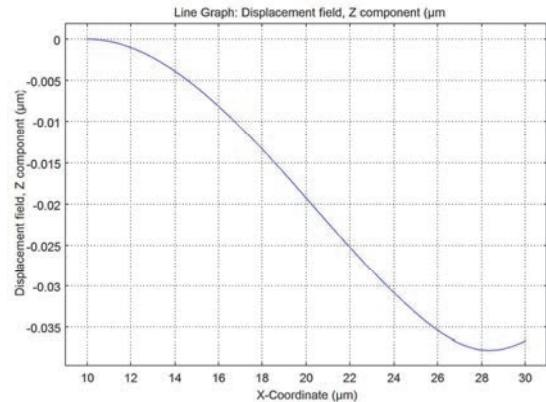
**Figure 8:** Z axis displacement field in the thinner membrane due to Electrostatic Force
