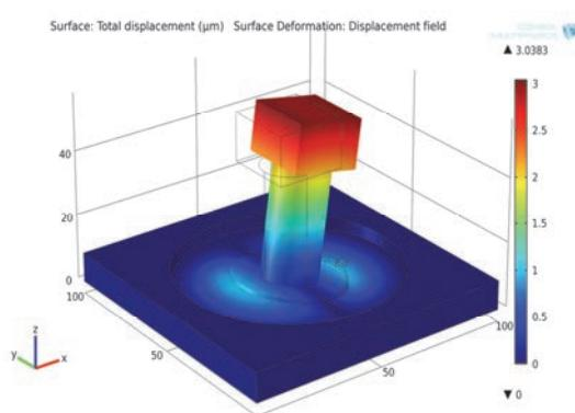
**Figure 7:** Displacement due to Coriolis Force in 3D model
