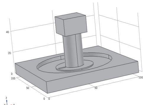
**Figure 5:** 3D Model of MEMS based Vibrating Gyroscope
