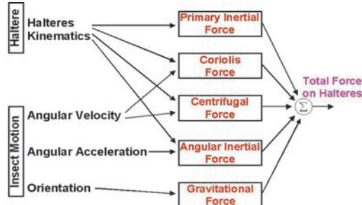
Figure 3: Haltere Force Modulation[2]
