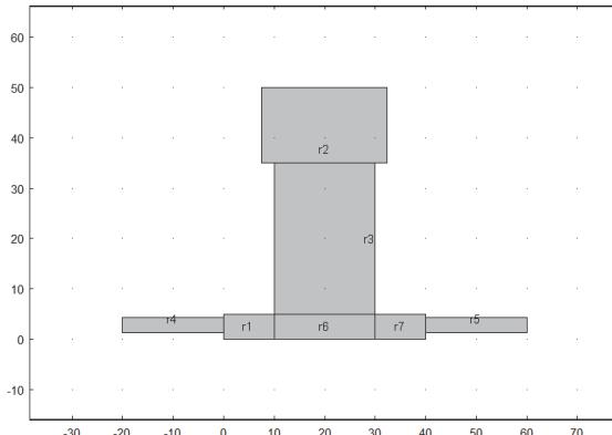
**Figure 4:** 2D Model of MEMS based Vibrating Gyroscope
