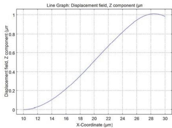
**Figure 9:** Z axis displacement field in the thinner membrane due to Coriolis Force
