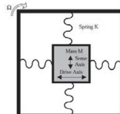
**Figure 1:** Basic Vibrational Gyroscope
