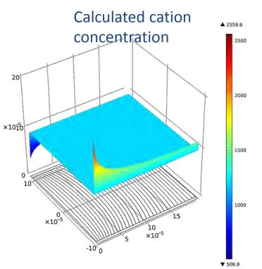
Cation concentration is projected on a full scale domain to calculate deformation
