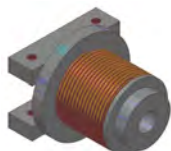
Figure 4. The construction of the coil module
