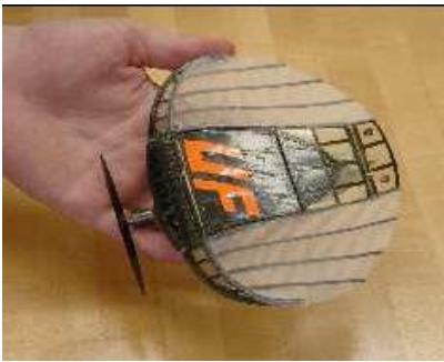
**Computational modeling of highly flexible membrane wings for MAVs**
