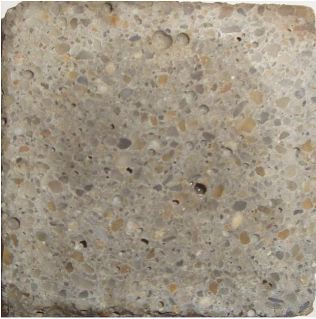
Figure 2: Air bubbles in mortar matrix
