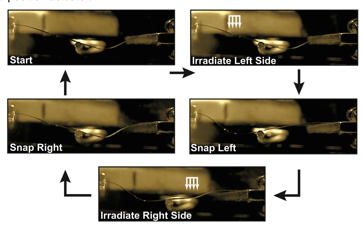
Light is used to drive left-right, fast, snap buckling in arches utilizing a third contact point positioned near the arch midpoint. The actuator operates on the principle of storage and quick release of elastic energy. Once in an equilibrium configuration the actuator can hold its position without further energy input. The material shown is an azobenzene functionalized polyimide.
