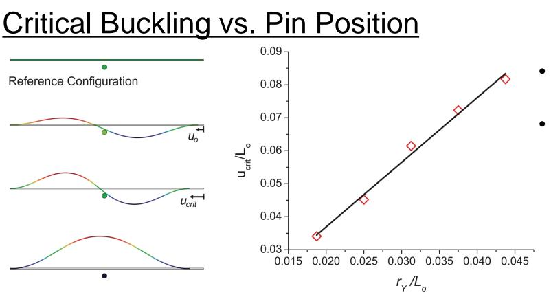
Critical displacement of the right end leads to pin contact, and rapid snap-through upward This data establishes a baseline linear trend for limits on end displacements suitable for photo-induced snap
