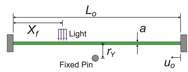
Inelastic Strains: Induced Photo-Strains
