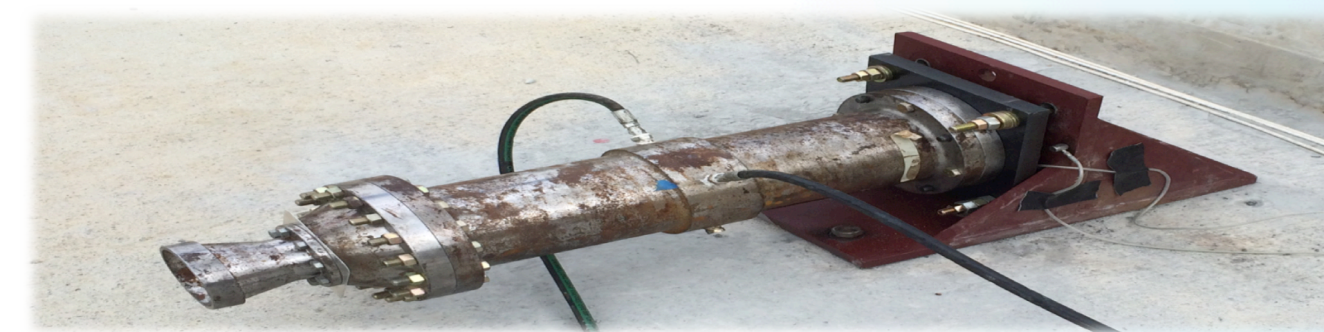
Figure 6. Cold Gas Thruster (CGT) used at the Portugues Dam
