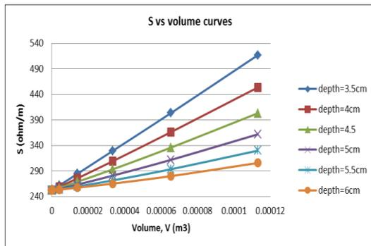
Figure 4: Relationship of  $S$  with object volume at different depth. The slope  $S$  is linearly proportional to the object volume  $V$ .
