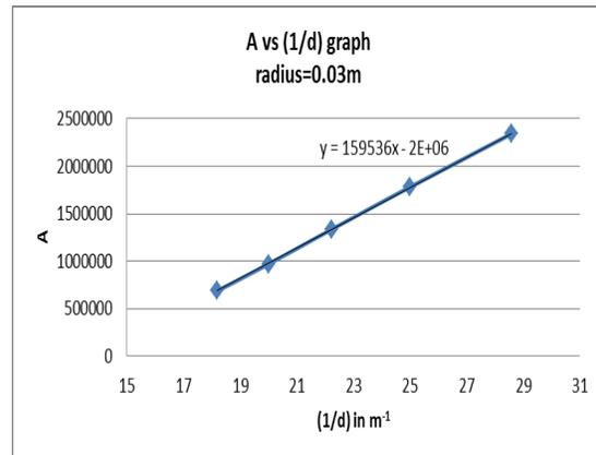
Figure 5: Relation between the slope  $A$  with object depth  $d$ . The slope  $A$  is inversely proportional to the depth.
