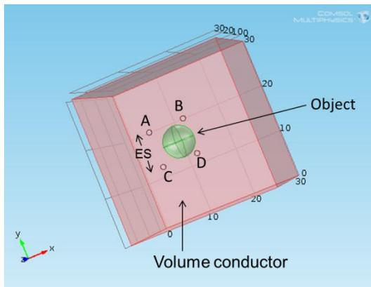
Figure 1: COMSOL model used in the volume determination study. A spherical object is embedded in a volume conductor. Electrodes are placed at the front surface of the volume conductor which is shown transparent.
