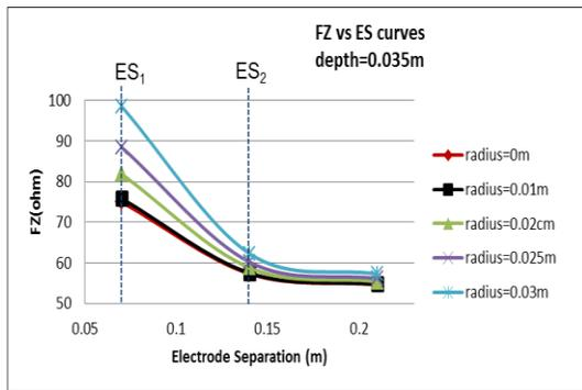
Figure 3: Change in Focused Impedance with increasing electrode separation for objects of different radius ( $r=0$  means no object). The object depth and conductivity were kept constant
