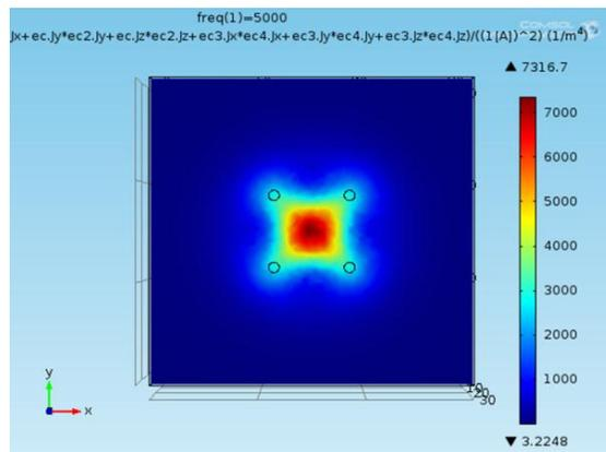
Figure 2: Sensitivity distribution of FIM at a plane at 3cm depth from the electrode plane showing enhanced sensitivity at the central zone.
