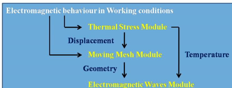
Figure 2. Computation Logical Diagram.
