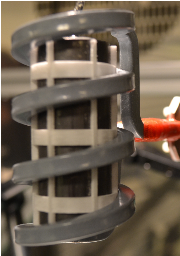
Figure 1: Experimental setup for Cylindrical cells. A special jig centers the cell inside the induction coil.
