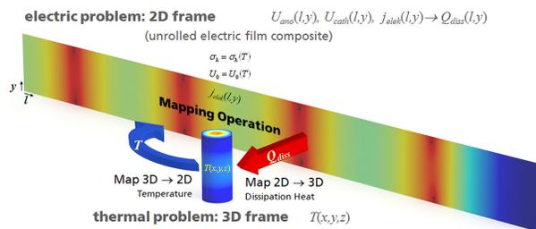
**Figure 2:** Hybrid 2D-3D-model approach with a 2D electric (unrolled winding body) and a 3D thermal branch (3D composite). Information is passed between the models during solution by a mapping process.
