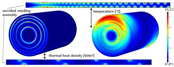
**Figure 4:** 2D and 3D Results (and its mappings) from the model for distribution of thermal heat density and temperature. Hot spots originate from the positions of the embedded contact tabs.
