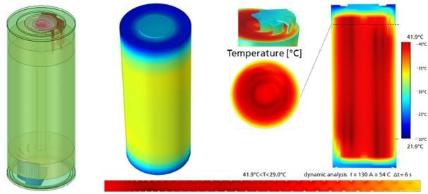
**Figure 3:** Results for the model of the complete cell with housing.
