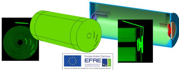
**Figure 1:** Example geometry of a Li-Ion-Cell: winding body with embedded contact tabs connected to housing and contacting structure
