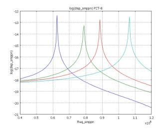
Figure 3: Mechanical resonance (displacement in log scale) of PZT-8.
