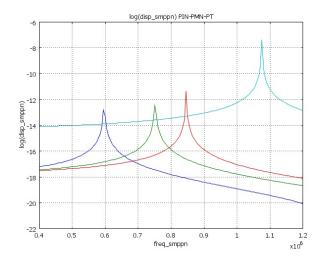
Figure 2: Mechanical resonance (displacement in log scale) of PIN-PMN-PT.
