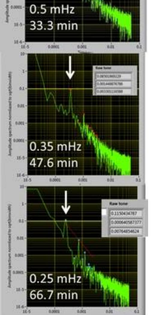
Figure 3. By varying the excitation frequency and measuring the instrument response in the Fourier domain (A), the system transfer function was experimentally determined (B red), and modeled for comparison (B blue).
