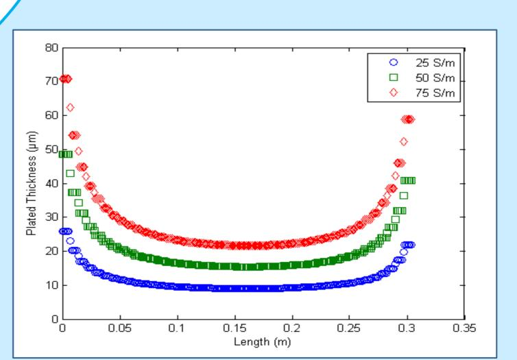
Plating thickness is directly proportional to solution conductivity however it also increases non-uniformity at higher values.
