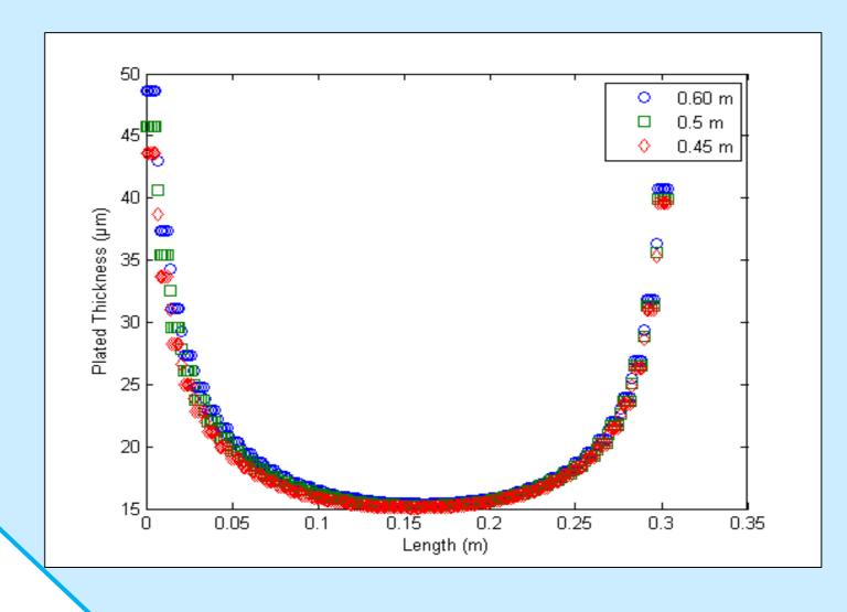
Anode height appears to have little effect on plating. Further refinement of the model is required to incorporate process sensitivity to this parameter.
