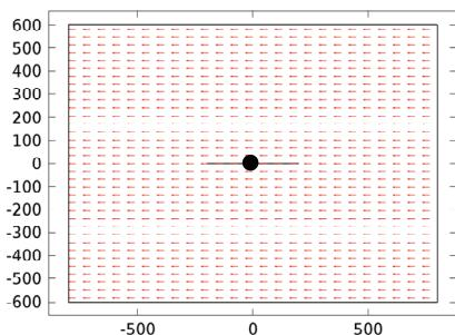
**Figure 6.** Initial maximum principle stress direction
