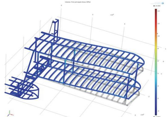
**Figure 7:** First principal stress for the flyer with two struts removed, as obtained from COMSOL.
