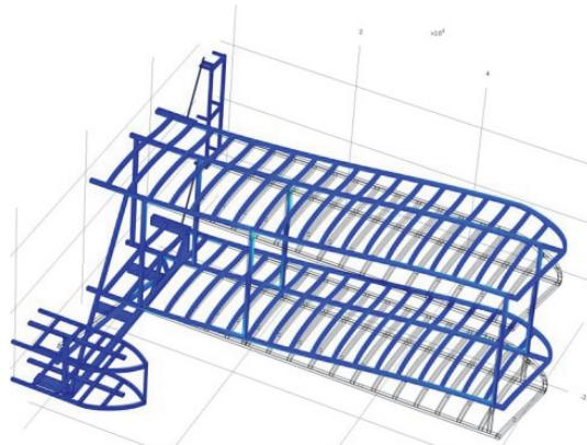
**Figure 4:** Modified flyer model with four struts removed
