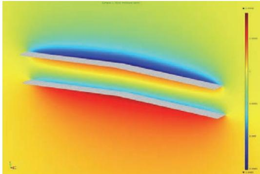
**Figure 4:** The pressure distribution on the two wings obtained from COMSOL.
