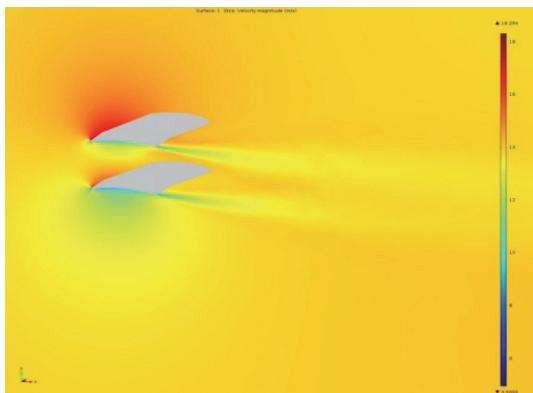
**Figure 5:** The velocity profile on the two wings obtained from COMSOL.
