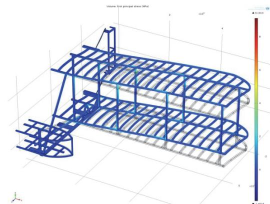
**Figure 6:** First principal stress for the flyer with the original 8 struts, as obtained from COMSOL.
