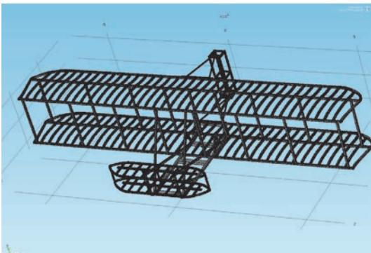
**Figure 3:** The original Wright brother's was meshed using COMSOL. Over a million DOF.
