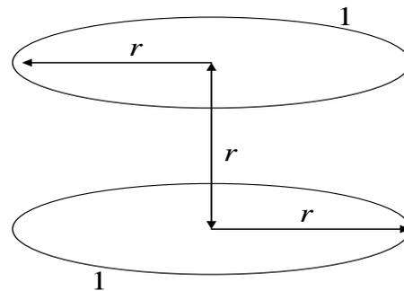
**Figure 1.** Helmholtz system coil.
