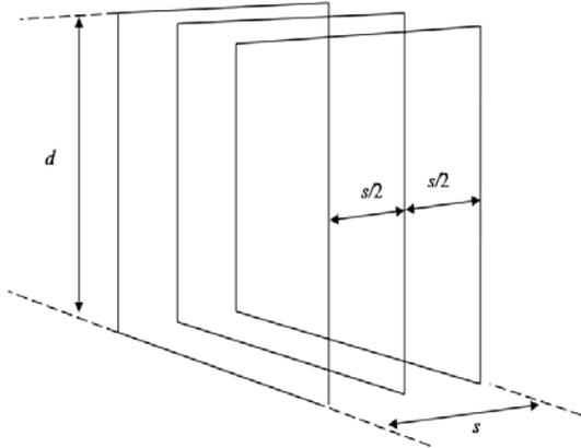
**Figure 2.** Merritt coil system -three square coils.
